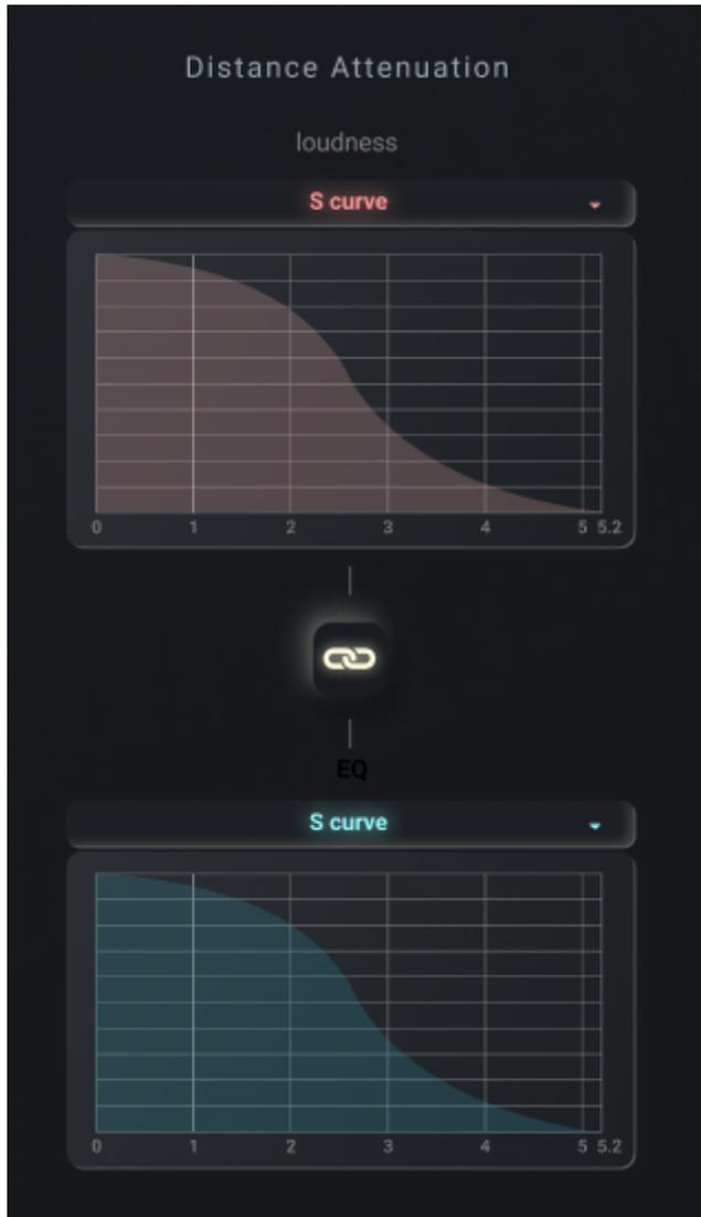
You can control the curve of distance attenuation. The volume of **Gain** decreases according to the distance from the center. The **EQ** suppresses high frequencies above 4kHz depending on the distance from the center.
