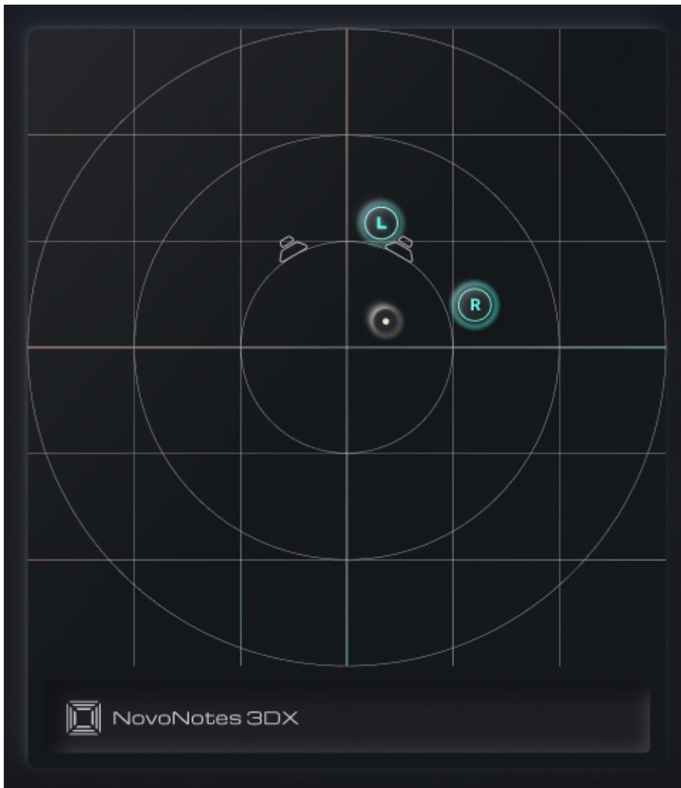
You can adjust the front / back and left / right positions of the sound source. When using Ambisonic for input, the entire sound field can be rotated.
